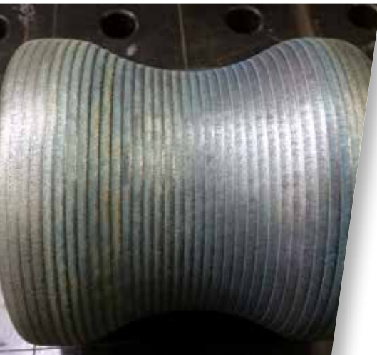
Smooth surface after Cladding
