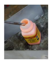
Manufactured in our brazing manufacturing plant in Villebonsur-Yvette (France), GreenFlux 1600 PF Atmosin is a complex salt mix of potassium fluoroborates and contains no boric acid or borax. It is intended for capillary brazing using high silver alloys. This brazing flux works on copper, bronze, brass, steel and stainless steel.
