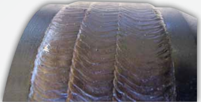
OTW 10SS hardbanding alloy applied on a tool-joint
