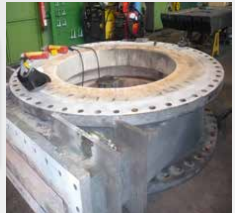
Hot wind valve blast furnace (FAR 2891)
